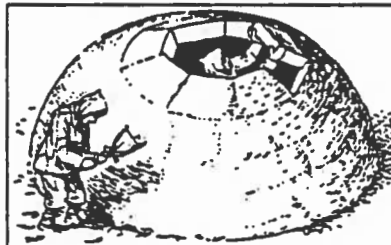
Finishing the house, the builder sets the last blocks in place as his wife plasters the exterior wall with soft snow.
